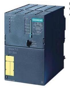
\*\*\* SPARE PART\*\*\* SIMATIC S7-300, CPU 317F-2DP, CENTRAL PROCESSING UNIT WITH 1024 KBYTE WORKING MEMORY, 1. INTERFACE MPI/DP 12MBIT/S, 2. INTERFACE DP-MASTER/SLAVE, MICRO MEMORY CARD NECESSARY FOR USE WITH SOFTWARE OPTION S7 DISTRIBUTED SAFETY V5.2 SP1 AND HIGHER
