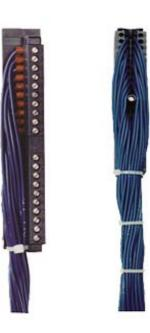
S7-300 FRONT CO. W. SINGLE CORES 3.2 M Front connector for SIMATIC S7-300, 20pole(6ES7392-1AJ00-0AA0) with 20 single cores 0.5 mm2, H05V-K single cores, screw-type version pack. unit = 1 piece, L = 3.2 m
